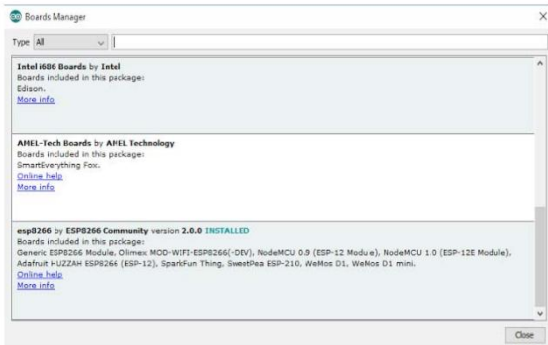
Figure 9: ESP 8266 board installation in Arduino
